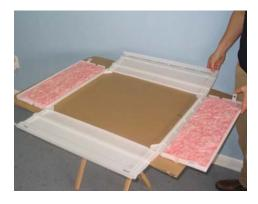
5. Lay the two long sides flat. Make sure to snap the flaps on the long sides shut.
